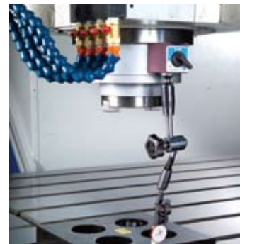
c. Geometric accuracy inspection ISO 10791-2
